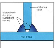
SGM steel wall sleeves are fitted with an anchoring collar **welded on right round and on both sides** (see diagramm).
