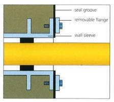
SGM sleeves with removable flanges provide a perfect water sealing when installed in seal grooves.
