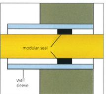
SGM fibre-cement wall sleeves are excellent for use with concrete. Their grooved exterior surface and homogenous material ensures the total join.
