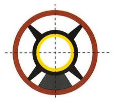
■ SGM pipe supports can centralize the carrier pipe in the casing and prevent the direct contact between the two pipes
