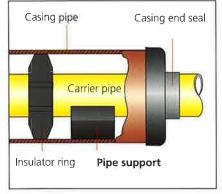
■ The thickness of the SGM pipe supports is coordinated to the available skid heights of SGM insulator segments
