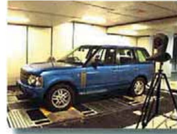
Acoustic measurement room with 4 WD Chassis Dynamometer; HEAD acoustics, Aachen, Germany
