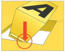
■ The bevelled edges of the fastening clip centres each piece on its insertion and ensures a flush fit to the next. (see drawing)
