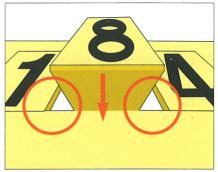
■ The barb of the fastening clip locks onto the corresponding rim of the sign plate.
